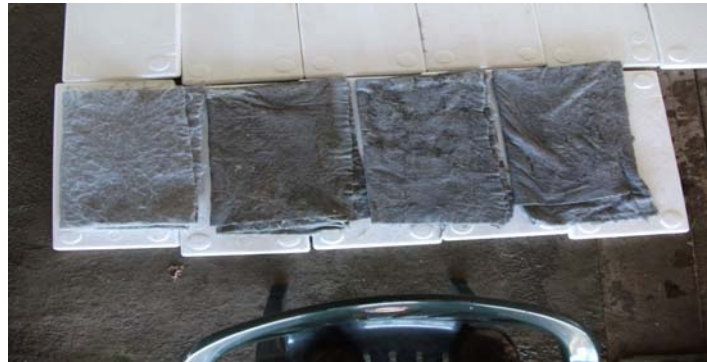
Fig 9 Mat filters used during purging. A) Bottom Dam B) Top Dam
